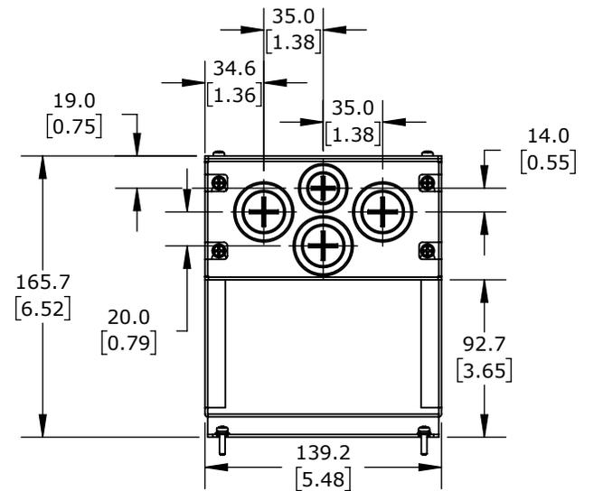
IRONHORSE ACG SERIES CONDUIT BOX, NEMA 1, FOR USE WITH ACG SERIES C FRAME AC DRIVES, MOUNTING HARDWARE INCLUDED
