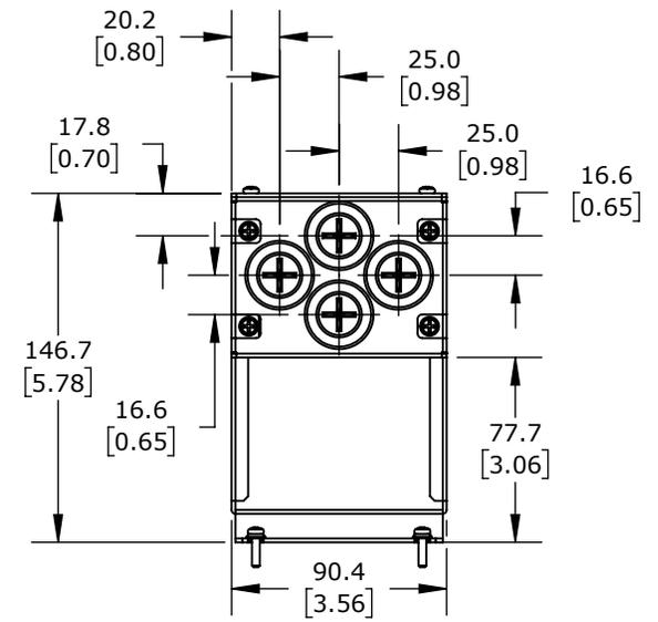
IRONHORSE ACG SERIES CONDUIT BOX, NEMA 1, FOR USE WITH ACG SERIES A FRAME AC DRIVES, MOUNTING HARDWARE INCLUDED
