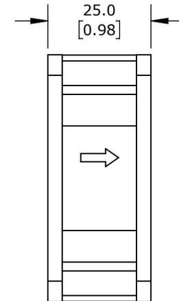
IRONHORSE ACG SERIES MAIN COOLING FAN, REPLACEMENT, 60 X 60 X 25mm, 24 VDC, FOR USE WITH ACG SERIES 7-1/2HP - 10HP AC DRIVES
