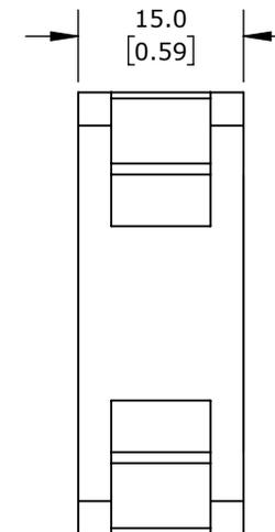
IRONHORSE ACG SERIES MAIN COOLING FAN, REPLACEMENT, 40 X 40 X 15mm, 24 VDC, FOR USE WITH ACG SERIES 1/2HP - 1HP AC DRIVES
