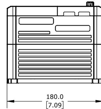
IRONHORSE ACG SERIES AC GENERAL PURPOSE DRIVE, ENCLOSED, 460 VAC, 7-1/2HP WITH 3-PHASE INPUT, 3HP WITH 1-PHASE INPUT, SVC OR V/Hz MODE, D FRAME, RS-485, MODBUS, 100KA SCCR. OPTIONAL ETHERNET/IP AND MODBUS TCP CARD AVAILABLE
