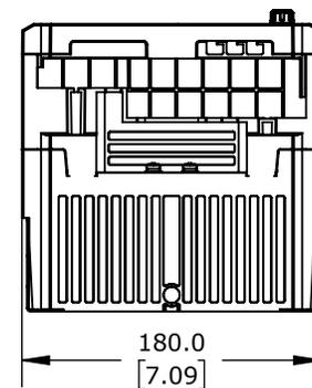
IRONHORSE ACG SERIES AC GENERAL PURPOSE DRIVE, ENCLOSED, 460 VAC, 15HP WITH 3-PHASE INPUT, 7-1/2HP WITH 1-PHASE INPUT, SVC OR V/Hz MODE, E FRAME, RS-485, MODBUS, 100KA SCCR. OPTIONAL ETHERNET/IP AND MODBUS TCP CARD AVAILABLE
