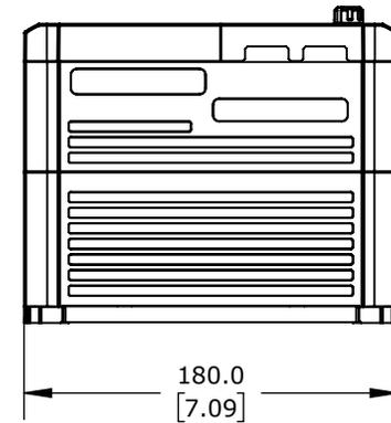
IRONHORSE ACG SERIES AC GENERAL PURPOSE DRIVE, ENCLOSED, 460 VAC, 10HP WITH 3-PHASE INPUT, 5HP WITH 1-PHASE INPUT, SVC OR V/Hz MODE, D FRAME, RS-485, MODBUS, 100KA SCCR. OPTIONAL ETHERNET/IP AND MODBUS TCP CARD AVAILABLE
