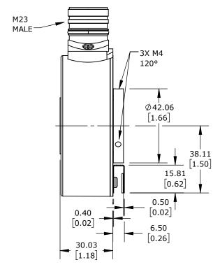
LIKA ELECTRONIC A80 SERIES INCREMENTAL (QUADRATURE) ROTARY ENCODER, MEDIUM DUTY, 5-30 VDC, RADIAL EXIT, UNIVERSAL (LINE DRIVER OR NPN/PNP OPEN COLLECTOR) OUTPUT, 1024 PPR, MULTIPLE SHAFTS (5/8IN - 30mm), 80mm DIAMETER BODY, IP64, M23 MALE
