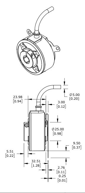
LIKA ELECTRONIC A50 SERIES INCREMENTAL (QUADRATURE) ROTARY ENCODER, MEDIUM DUTY, 5-30 VDC, RADIAL EXIT, UNIVERSAL (LINE DRIVER OR NPN/PNP OPEN COLLECTOR) OUTPUT, 1024 PPR, 3/8IN HOLLOW SHAFT, 50mm DIAMETER BODY, IP65, 6.5FT/2M CABLE LENGTH, PIGTAIL
