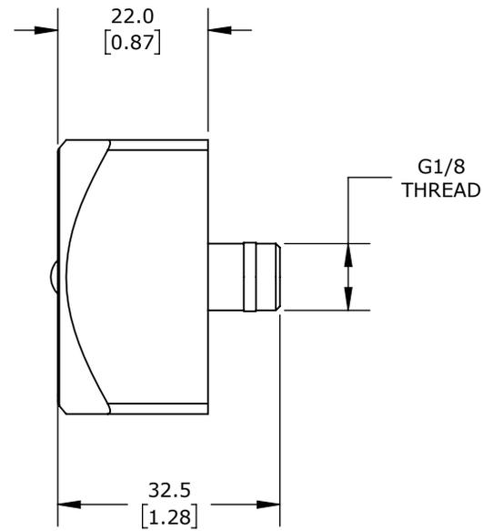
**METAL WORK PNEUMATIC PRESSURE GAUGE**
