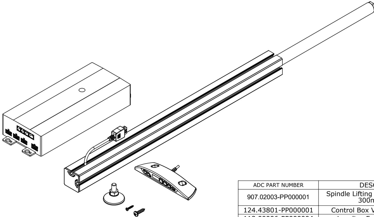
300mm STROKE, 1100 LBS/500 KG. FOR USE WITH 40 X 40mm
