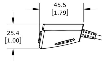
MANUAL SWITCH, IP30. FOR USE WITH ERGOSWISS 124.43800-PP000001 AND 124.43801-PP000001 CONTROL BOXES. (1) 6.5FT/2.0M POWER CABLE INCLUDED. SAVES (3) INTERMEDIATE POSITIONS IN ADDITION TO UP AND DOWN FUNCTION.
