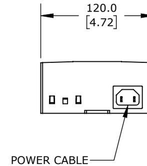
110 VAC NOMINAL INPUT, 24 VAC, IP20. FOR USE WITH UP TO (4) ERGOSWISS 907.02003-PP000001 SPINDLE LIFTING COLUMNS.
