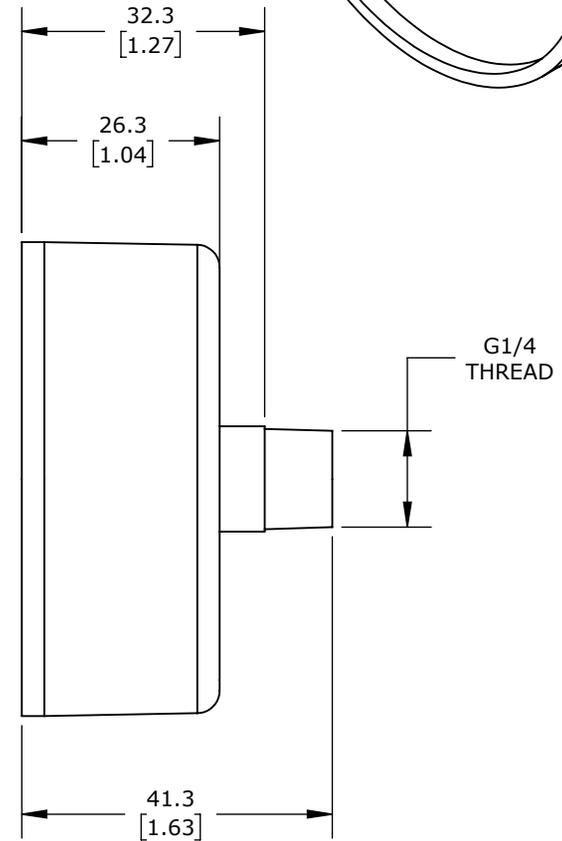
**METAL WORK PNEUMATIC PRESSURE GAUGE**
