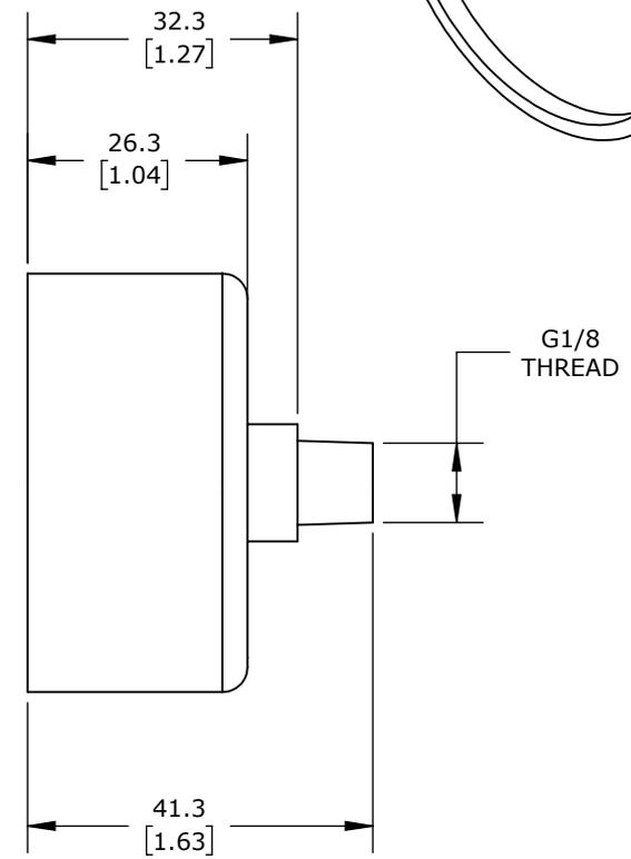
**METAL WORK PNEUMATIC PRESSURE GAUGE**
