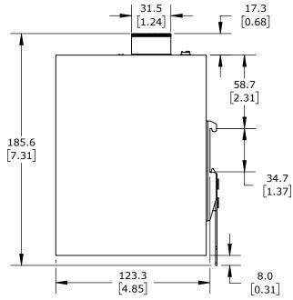
WAGO INDUSTRIAL LEAN MANAGED ETHERNET SWITCH, 16 PORTS, (16) ETHERNET GIGABIT (RJ45) PORT(s), MODBUS TCP AND SNMP, -40 TO +60 DEG C, METAL HOUSING, IP30, 35mm DIN RAIL MOUNT
