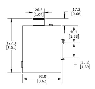
WAGO INDUSTRIAL LEAN MANAGED ETHERNET SWITCH, MAC SECURITY, 8 PORTS, (6) ETHERNET GIGABIT (RJ45) AND (2) SFP COMBO GIGABIT PORT(s), MODBUS TCP AND SNMP, -20 TO +70 DEG C, METAL HOUSING, IP30, 35mm DIN RAIL MOUNT
