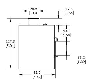
WAGO INDUSTRIAL LEAN MANAGED ETHERNET SWITCH, MAC SECURITY, 8 PORTS, (8) ETHERNET GIGABIT (RJ45) PORT(s), MODBUS TCP AND SNMP, -20 TO +70 DEG C, METAL HOUSING, IP30, 35mm DIN RAIL MOUNT
