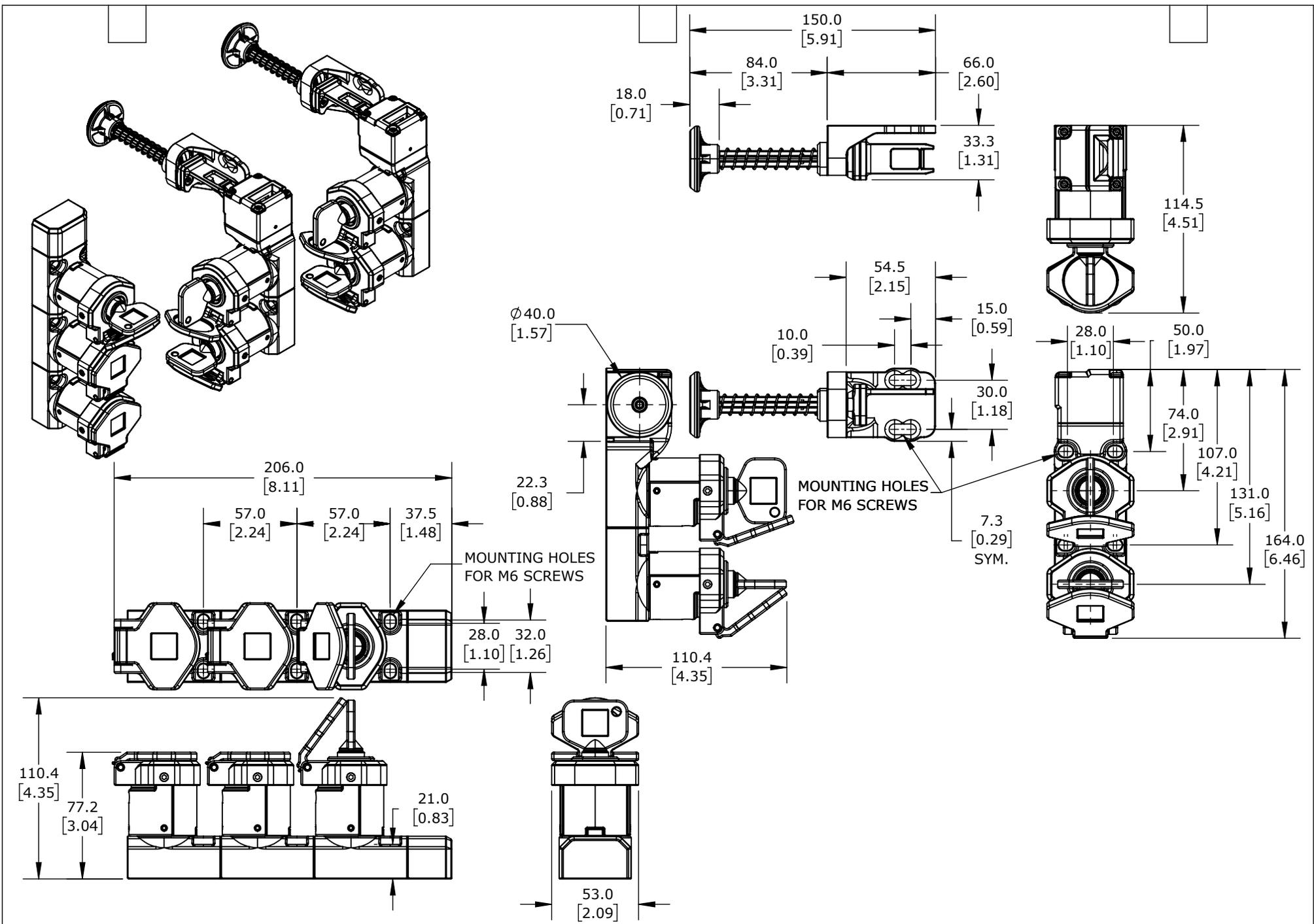
IDEM SKORPION SERIES TRAPPED KEY INTERLOCK SYSTEM, ROTARY KEY, 2 GATES, WHOLE BODY, A103 CODED, DIE-CAST ALUMINUM ALLOY.
