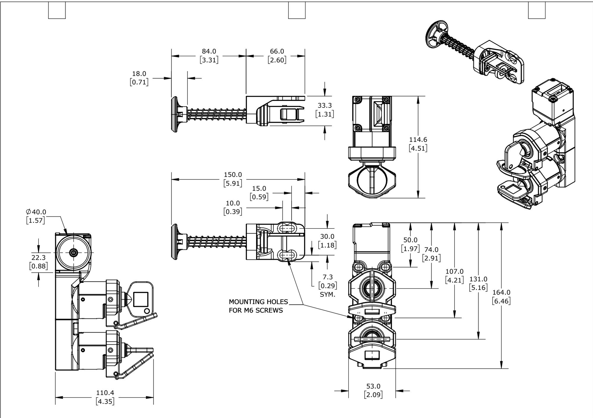
IDEM SKORPION SERIES TRAPPED KEY INTERLOCK SYSTEM, ROTARY KEY, 1 GATE, WHOLE BODY, A104 CODED, DIE-CAST ALUMINUM ALLOY.
