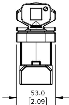
IDEM SKORPION SERIES TRAPPED KEY INTERLOCK SYSTEM, ROTARY KEY, 2 GATES, PARTIAL BODY, A103 CODED, DIE-CAST ALUMINUM ALLOY.
