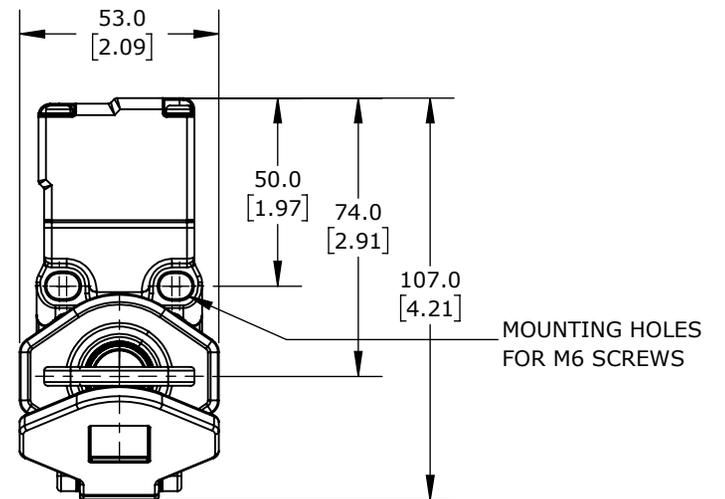
IDEM SKORPION SERIES TRAPPED KEY INTERLOCK SYSTEM, ROTARY KEY, 1 GATE, PARTIAL BODY, A103 CODED, DIE-CAST ALUMINUM ALLOY.
