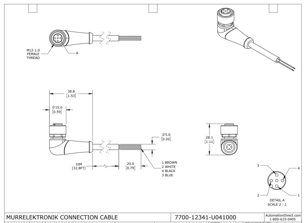
3rd NOT TO PART DIMENSIONS MAY DIFFER SLIGHTLY METRIC UNITS USED UNLESS OTHERWISE **mm** MODEL ANGLE SCALE DUE TO MANUFACTURER'S VARIANCES FOR PART DESIGN SPECIFIED UNITS ARE: **[inch]** REV. - DRAWING DATE 6/4/2025 SHEET 1 OF 1
