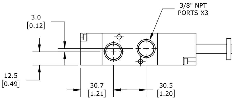
3-PORT (3-WAY), 2-POSITION, N.C., SINGLE SOLENOID SPRING RETURN, 3/8IN FEMALE NPT INLET(S), 3/8IN FEMALE NPT OUTLET(S), 3/8IN FEMALE NPT EXHAUST(S), 1/8IN FEMALE NPT PILOT(S), CV=2.1.
