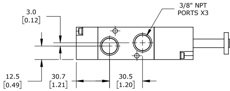
3-PORT (3-WAY), 2-POSITION, N.O., SINGLE SOLENOID SPRING RETURN, 3/8IN FEMALE NPT INLET(S), 3/8IN FEMALE NPT OUTLET(S), 3/8IN FEMALE NPT EXHAUST(S), CV=2.1.
