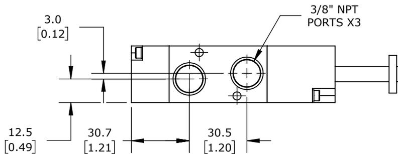
3-PORT (3-WAY), 2-POSITION, N.C., SINGLE SOLENOID SPRING RETURN, 3/8IN FEMALE NPT INLET(S), 3/8IN FEMALE NPT OUTLET(S), 3/8IN FEMALE NPT EXHAUST(S), CV=2.1.
