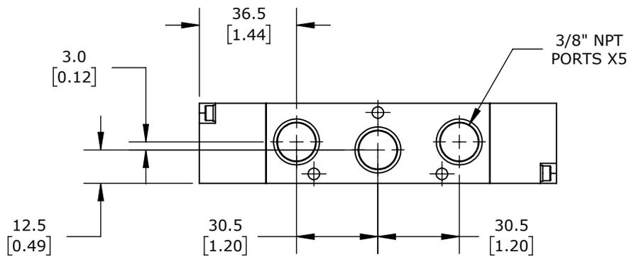
5-PORT (4-WAY), 2-POSITION, DOUBLE AIR PILOT, 3/8IN FEMALE NPT INLET(S), 3/8IN FEMALE NPT OUTLET(S), 3/8IN FEMALE NPT EXHAUST(S), 1/8IN FEMALE NPT PILOT(S), CV=2.1.
