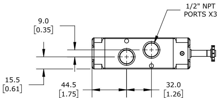
3-PORT (3-WAY), 2-POSITION, N.C., SINGLE SOLENOID SPRING RETURN, 1/2IN FEMALE NPT INLET(S), 1/2IN FEMALE NPT OUTLET(S), 1/2IN FEMALE NPT EXHAUST(S), 1/8IN FEMALE NPT PILOT(S), CV=4.6.
