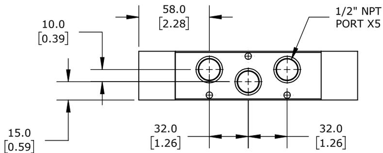
5-PORT (4-WAY), 3-POSITION, CENTER CLOSED, DOUBLE AIR PILOT, 1/2IN FEMALE NPT INLET(S), 1/2IN FEMALE NPT OUTLET(S), 1/2IN FEMALE NPT EXHAUST(S), 1/8IN FEMALE NPT PILOT(S), CV=4.6.
