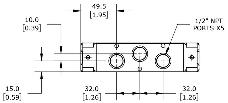
5-PORT (4-WAY), 2-POSITION, DOUBLE AIR PILOT, 1/2IN FEMALE NPT INLET(S), 1/2IN FEMALE NPT OUTLET(S), 1/2IN FEMALE NPT EXHAUST(S), 1/8IN FEMALE NPT PILOT(S), CV=4.6.
