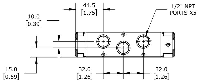
5-PORT (4-WAY), 2-POSITION, SINGLE AIR PILOT SPRING RETURN, 1/2IN FEMALE NPT INLET(S), 1/2IN FEMALE NPT OUTLET(S), 1/2IN FEMALE NPT EXHAUST(S), 1/8IN FEMALE NPT PILOT(S), CV=4.6.
