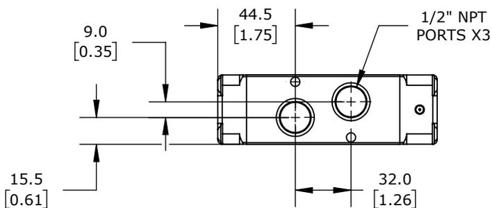
3-PORT (3-WAY), 2-POSITION, N.C., SINGLE AIR PILOT SPRING RETURN, 1/2IN FEMALE NPT INLET(S), 1/2IN FEMALE NPT OUTLET(S), 1/2IN FEMALE NPT EXHAUST(S), 1/8IN FEMALE NPT PILOT(S), CV=4.6.
