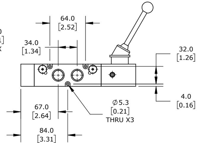
5-PORT (4-WAY), 3-POSITION, CENTER EXHAUST, 90 DEG HAND LEVER, DETENTED, 1/2IN FEMALE NPT INLET(S), 1/2IN FEMALE NPT OUTLET(S), 1/2IN FEMALE NPT EXHAUST(S), CV=4.6.
