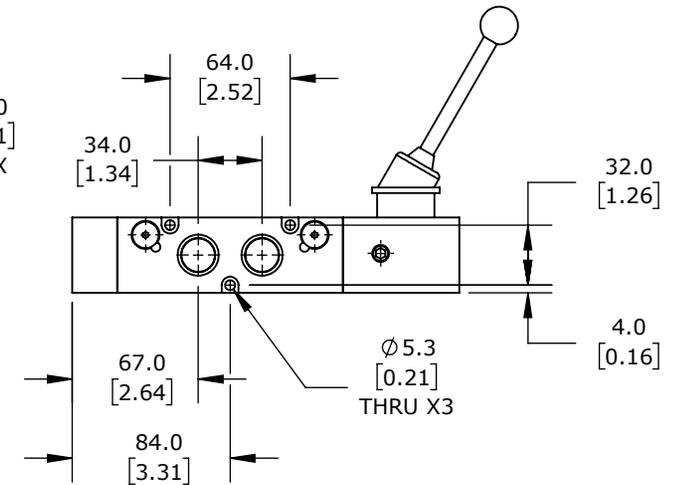
5-PORT (4-WAY), 2-POSITION, 90 DEG HAND LEVER, SPRING RETURN, 1/2IN FEMALE NPT INLET(S), 1/2IN FEMALE NPT OUTLET(S), 1/2IN FEMALE NPT EXHAUST(S), CV=4.6.
