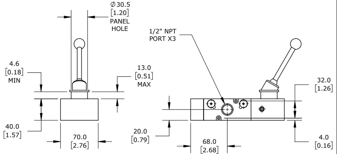
3-PORT (3-WAY), 2-POSITION, 90 DEG HAND LEVER, DETENTED,
