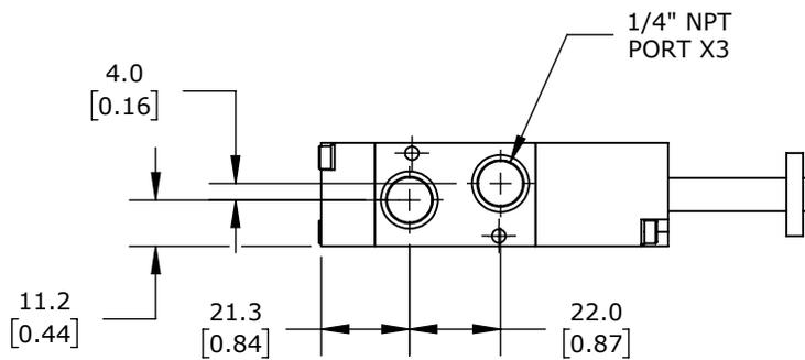
3-PORT (3-WAY), 2-POSITION, N.C., SINGLE SOLENOID SPRING RETURN, 1/4IN FEMALE NPT INLET(S), 1/4IN FEMALE NPT OUTLET(S), 1/4IN FEMALE NPT EXHAUST(S), CV=1.1.
