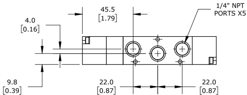
5-PORT (4-WAY), 3-POSITION, CENTER PRESSURE, DOUBLE AIR PILOT, 1/4IN FEMALE NPT INLET(S), 1/4IN FEMALE NPT OUTLET(S), 1/4IN FEMALE NPT EXHAUST(S), 1/8IN FEMALE NPT PILOT(S), CV=1.1.
