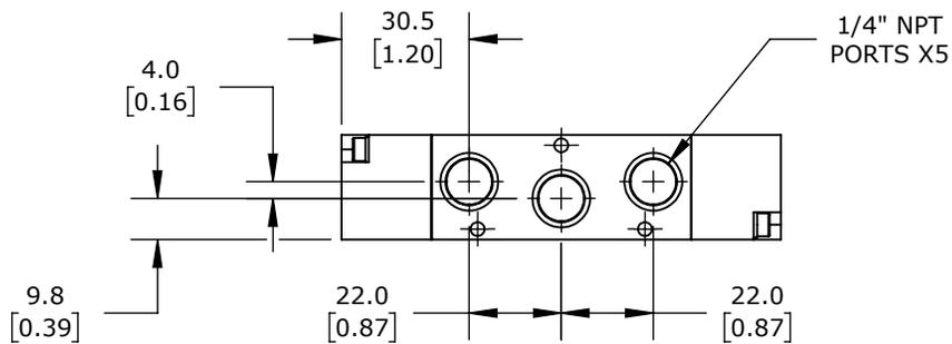
5-PORT (4-WAY), 2-POSITION, DOUBLE AIR PILOT, 1/4IN FEMALE NPT INLET(S), 1/4IN FEMALE NPT OUTLET(S), 1/4IN FEMALE NPT EXHAUST(S), 1/8IN FEMALE NPT PILOT(S), CV=1.1.
