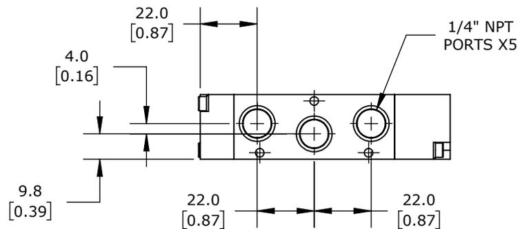
5-PORT (4-WAY), 2-POSITION, SINGLE AIR PILOT SPRING RETURN, 1/4IN FEMALE NPT INLET(S), 1/4IN FEMALE NPT OUTLET(S), 1/4IN FEMALE NPT EXHAUST(S), 1/8IN FEMALE NPT PILOT(S), CV=1.1.
