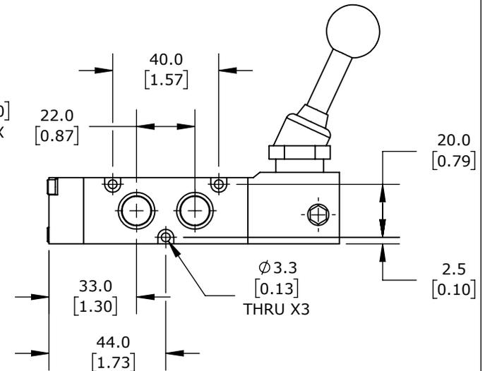
5-PORT (4-WAY), 2-POSITION, 90 DEG HAND LEVER, DETENTED, 1/4IN FEMALE NPT INLET(S), 1/4IN FEMALE NPT OUTLET(S), 1/4IN FEMALE NPT EXHAUST(S), CV=1.1.
