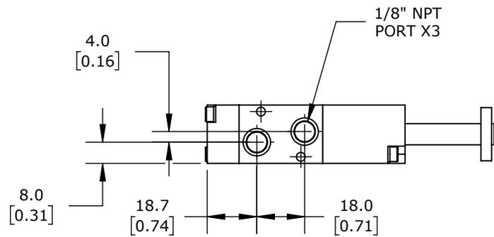
3-PORT (3-WAY), 2-POSITION, N.C., SINGLE SOLENOID SPRING RETURN, 1/8IN FEMALE NPT INLET(S), 1/8IN FEMALE NPT OUTLET(S), 1/8IN FEMALE NPT EXHAUST(S), #10-32 FEMALE UNF PILOT(S), CV=0.55
