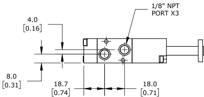
3-PORT (3-WAY), 2-POSITION, N.O., SINGLE SOLENOID SPRING RETURN, 1/8IN FEMALE NPT INLET(S), 1/8IN FEMALE NPT OUTLET(S), 1/8IN FEMALE NPT EXHAUST(S), CV=0.55.
