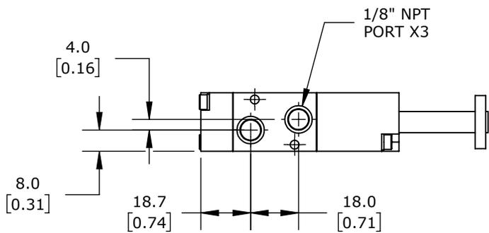
3-PORT (3-WAY), 2-POSITION, N.C., SINGLE SOLENOID SPRING RETURN, 1/8IN FEMALE NPT INLET(S), 1/8IN FEMALE NPT OUTLET(S), 1/8IN FEMALE NPT EXHAUST(S), CV=0.55.
