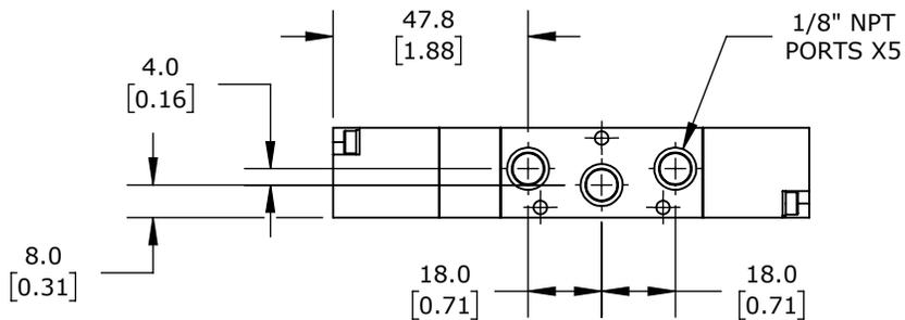
5-PORT (4-WAY), 3-POSITION, CENTER PRESSURE, DOUBLE AIR PILOT,
