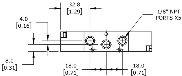
5-PORT (4-WAY), 2-POSITION, DOUBLE AIR PILOT, 1/8IN FEMALE NPT INLET(S), 1/8IN FEMALE NPT OUTLET(S), 1/8IN FEMALE NPT EXHAUST(S), 1/8IN FEMALE NPT PILOT(S), CV=0.55.
