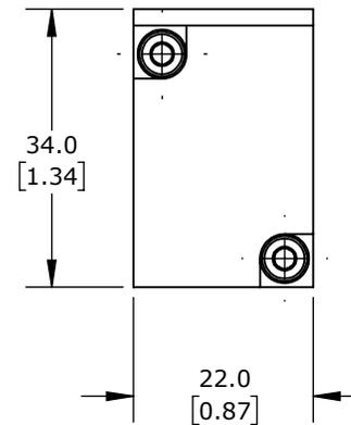
3-PORT (3-WAY), 2-POSITION, N.O., SINGLE AIR PILOT SPRING RETURN, 1/8IN FEMALE NPT INLET(S), 1/8IN FEMALE NPT OUTLET(S), 1/8IN FEMALE NPT EXHAUST(S), 1/8IN FEMALE NPT PILOT(S), CV=0.55.
