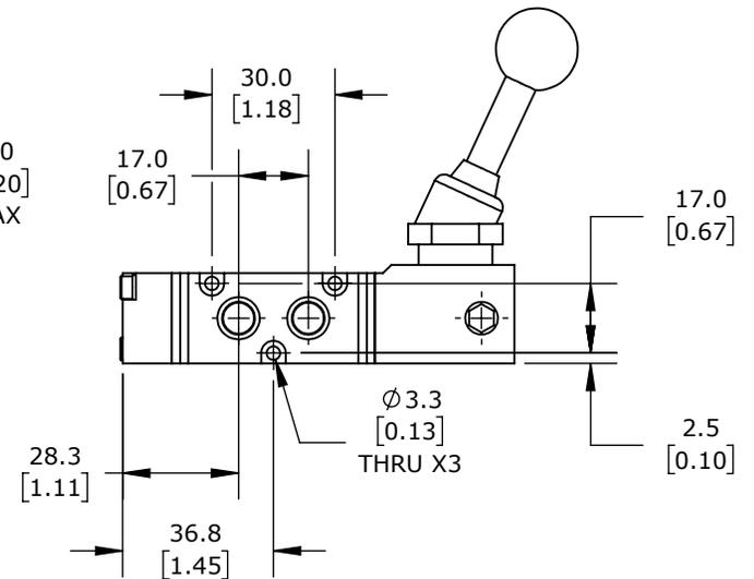
5-PORT (4-WAY), 3-POSITION, CENTER PRESSURE, 90 DEG HAND LEVER, SPRING RETURN, 1/8IN FEMALE NPT INLET(S), 1/8IN FEMALE NPT OUTLET(S), 1/8IN FEMALE NPT EXHAUST(S), CV=0.55.
