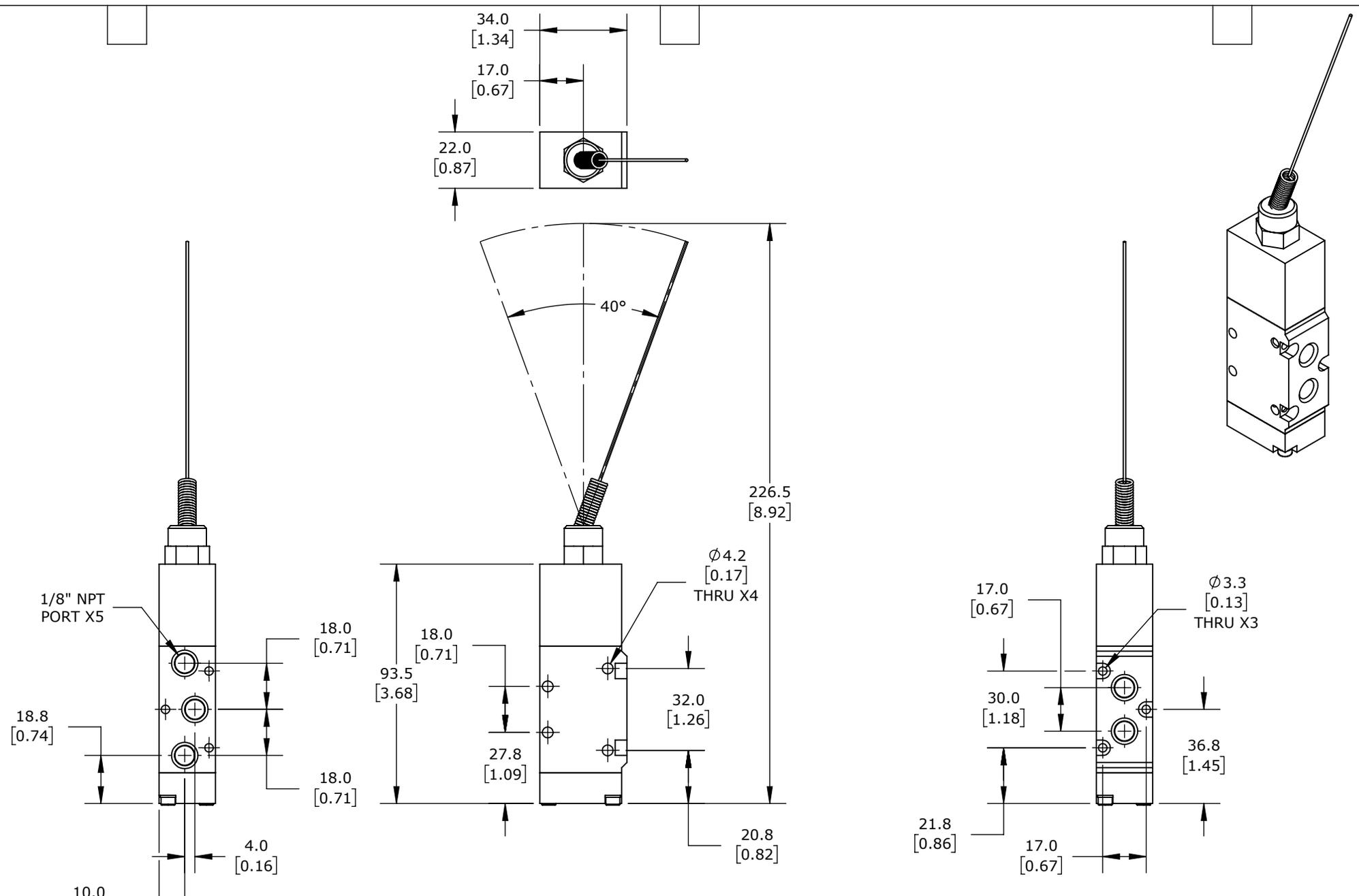
MECHANICALLY OPERATED DIRECTIONAL CONTROL VALVE, 5-PORT (4-WAY), 2-POSITION, PILOT-ASSISTED WHISKER, SPRING RETURN, 1/8IN FEMALE NPT INLET(S), 1/8IN FEMALE NPT OUTLET(S), 1/8IN FEMALE NPT EXHAUST(S), CV=0.55.
