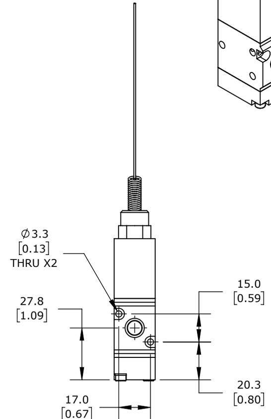
MECHANICALLY OPERATED DIRECTIONAL CONTROL VALVE, 3-PORT (3-WAY), 2-POSITION, N.C., PILOT-ASSISTED WHISKER, SPRING RETURN, 1/8IN FEMALE NPT INLET(S), 1/8IN FEMALE NPT OUTLET(S), 1/8IN FEMALE NPT EXHAUST(S), CV=0.55.
