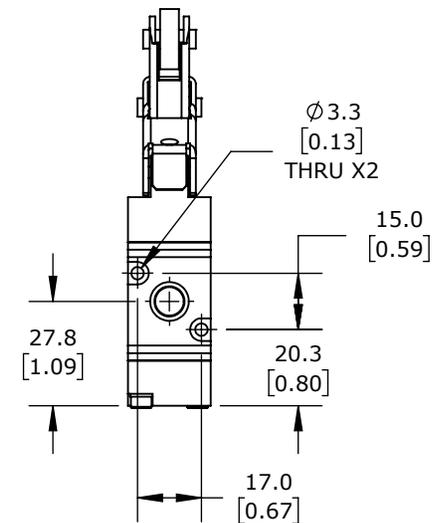
MECHANICALLY OPERATED DIRECTIONAL CONTROL VALVE, 3-PORT (3-WAY), 2-POSITION, N.C., UNIDIRECTIONAL ROLLER LEVER, SPRING RETURN, 1/8IN FEMALE NPT INLET(S), 1/8IN FEMALE NPT OUTLET(S), 1/8IN FEMALE NPT EXHAUST(S), CV=0.55.
