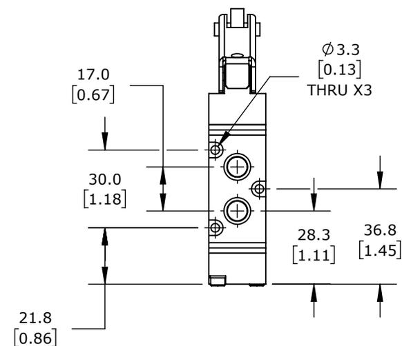
MECHANICALLY OPERATED DIRECTIONAL CONTROL VALVE, 5-PORT (4-WAY), 2-POSITION, ROLLER LEVER, SPRING RETURN, 1/8IN FEMALE NPT INLET(S), 1/8IN FEMALE NPT OUTLET(S), 1/8IN FEMALE NPT EXHAUST(S), CV=0.55.
