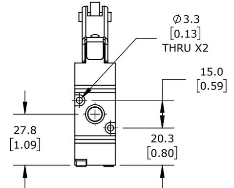
3-PORT (3-WAY), 2-POSITION, N.C., ROLLER LEVER, SPRING RETURN, 1/8IN FEMALE NPT INLET(S), 1/8IN FEMALE NPT OUTLET(S), 1/8IN FEMALE NPT EXHAUST(S), CV=0.55.
